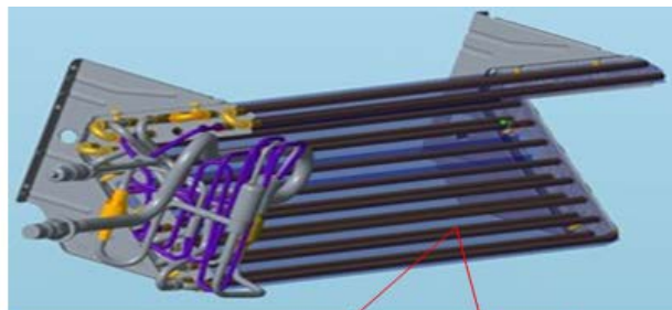
Video camera close-up V-type evaporator design
